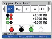
Isolation resistance measurement reveals damage to cable isolation, moisture penetration or oxidised contact points in the line. The subscriber line must show a resistance of 5 to 10  $M\Omega$  or more.
