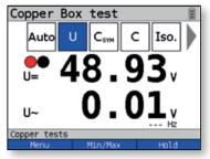
With DC/AC voltage measurement, you can verify that no external voltages are present (e.g. < 1 V), or whether supply voltages are connected.
