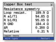
Loop resistance measurement enables you to detect short-circuits and estimate line lengths, among other things. Using resistive symmetry, you can also detect irregularities in the cable (e.g. too great difference in resistance) that can cause signal distortions and transmission errors.
