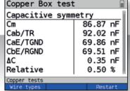
This function detects whether the line is open and determines the input capacitance of connected devices and the capacitance of the open line. With the aid of capacitive symmetry measurement (deviation < 1 %), it is possible to detect irregularities in the cable that can result in signal distortions or transmission errors.
