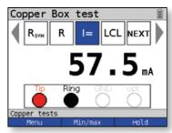
Use DC current measurement to verify that no leakage or external currents are flowing on the selected line (ideal: 0 mA).
